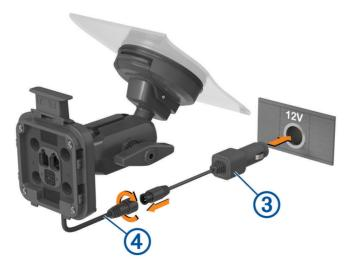
6 Tighten the collar around the connected power cables.
